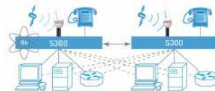
Redundant, resilient and secure configuration incorporating a Rubidium Oscillator in the primary server and peering to another server for backup redundancy.
