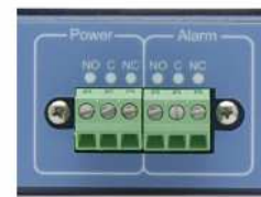
User configurable alarm relays for major/minor alarms as well loss-of-power alarm relay.
