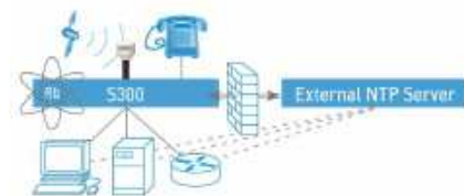
Resilient internal configuration. However, security, accuracy and reliability risks exist when peering with an external time server through the firewall.
