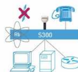
Resilient configuration incorporating a Rubidium Oscillator for improved holdover performance.
