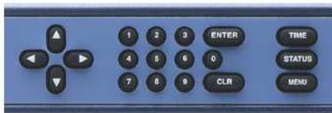
The full numeric keypad is the most efficient way to navigate a menu driven interface. The [TIME] & [STATUS] buttons quickly display the most critical information.
