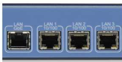
Four network ports (including Gigabit) provide network configuration flexibility and enhanced security. "Multiple" isolated and synchronized time servers can also be configured.
