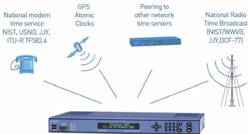
Internal modem and optional AM radio antenna provide access to national time sources for time reference redundancy.
