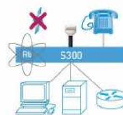
Resilient configuration incorporating a Rubidium Oscillator for improved holdover performance.
